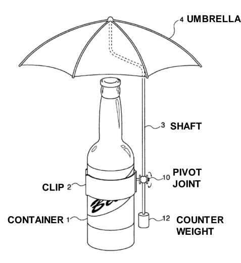
Clip 2 may be removably attached to container 1 such that the apparatus may be reused on another container when container 1 is empty. Attached to clip 2 is shaft 3 for supporting umbrella 4. Umbrella 4 may be fixed to shaft 3 or may be attached using a pivot joint or the like as will be discussed in more detail below. Shaft 3 may be made of plastic, wood, cardboard, or metal, but in the preferred embodiment is plastic.
